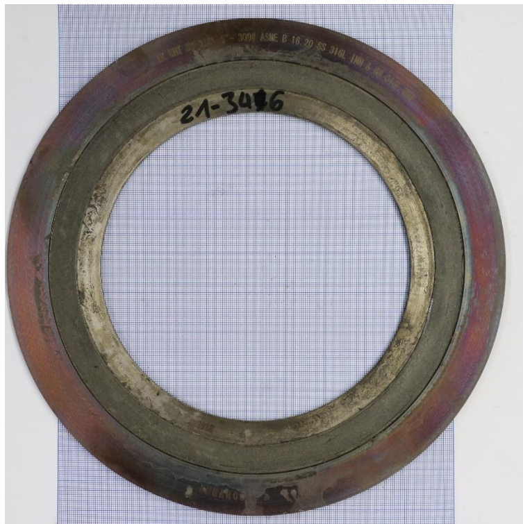
INMARCO - 1K UHT SS316L-SS316L Inn & SS316L OUT after Fire Test 21-346 according to API Specification 6FB
